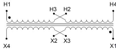
Single Phase Control Transformer with a capacity of 250VA, transforming 120/240 Volts to 12/24 Volts
