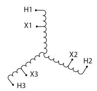
Three Phase Autotransformer with a capacity of 6kVA, transforming 110Y Volts to 575Y Volts
