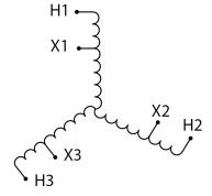
Three Phase Autotransformer with a capacity of 9kVA, transforming 200Y Volts to 480Y Volts
