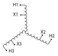
Three Phase Autotransformer with a capacity of 750kVA, transforming 120Y Volts to 400Y Volts
