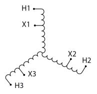
Three Phase Autotransformer with a capacity of 750kVA, transforming 480Y Volts to 115Y Volts
