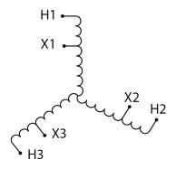
Three Phase Autotransformer with a capacity of 1500kVA, transforming 380Y Volts to 240Y Volts
