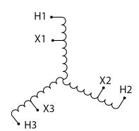
Three Phase Autotransformer with a capacity of 75kVA, transforming 440Y Volts to 110Y Volts
