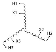
Three Phase Autotransformer with a capacity of 112.5kVA, transforming 110Y Volts to 400Y Volts
