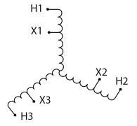
Three Phase Autotransformer with a capacity of 112.5kVA, transforming 110Y Volts to 550Y Volts
