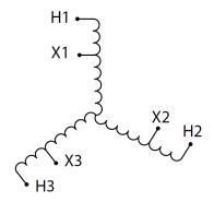
Three Phase Autotransformer with a capacity of 112.5kVA, transforming 115Y Volts to 240Y Volts
