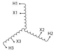
Three Phase Autotransformer with a capacity of 112.5kVA, transforming 115Y Volts to 416Y Volts
