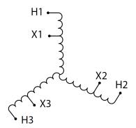
Three Phase Autotransformer with a capacity of 112.5kVA, transforming 200Y Volts to 550Y Volts
