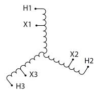
Three Phase Autotransformer with a capacity of 112.5kVA, transforming 480Y Volts to 230Y Volts
