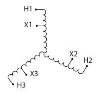
Three Phase Autotransformer with a capacity of 112.5kVA, transforming 575Y Volts to 110Y Volts
