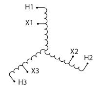
Three Phase Encapsulated Autotransformer with a capacity of 150kVA, transforming 480Y Volts to 208Y Volts
