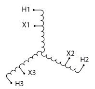
Three Phase Autotransformer with a capacity of 15kVA, transforming 200Y Volts to 550Y Volts
