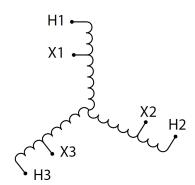
Three Phase Autotransformer with a capacity of 30kVA, transforming 120Y Volts to 416Y Volts
