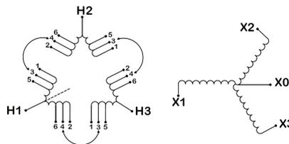
Three Phase Isolation Transformer with a capacity of 750kVA, transforming 600 Volts to 240Y/139 Volts
