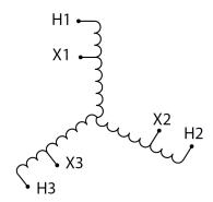
Three Phase Autotransformer with a capacity of 75kVA, transforming 460Y Volts to 120Y Volts
