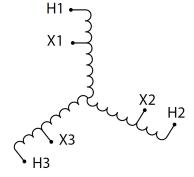
Three Phase Autotransformer with a capacity of 112.5kVA, transforming 200Y Volts to 208Y Volts
