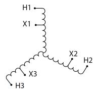
Three Phase Autotransformer with a capacity of 112.5kVA, transforming 200Y Volts to 240Y Volts
