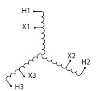
Three Phase Autotransformer with a capacity of 112.5kVA, transforming 400Y Volts to 347Y Volts
