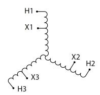
Three Phase Autotransformer with a capacity of 112.5kVA, transforming 600Y Volts to 347Y Volts
