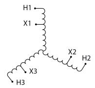
Three Phase Autotransformer with a capacity of 150kVA, transforming 220Y Volts to 416Y Volts
