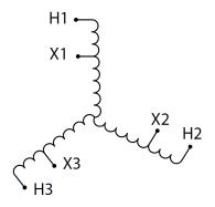
Three Phase Autotransformer with a capacity of 45kVA, transforming 550Y Volts to 115Y Volts
