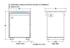
Three Phase Isolation Transformer with a capacity of 225kVA, transforming 600 Volts to 416Y/240 Volts
