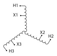
Three Phase Autotransformer with a capacity of 45kVA, transforming 550Y Volts to 208Y Volts
