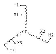
Three Phase Autotransformer with a capacity of 75kVA, transforming 240Y Volts to 347Y Volts
