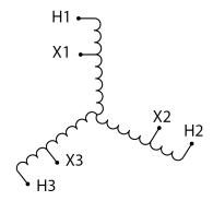
Three Phase Autotransformer with a capacity of 75kVA, transforming 347Y Volts to 240Y Volts
