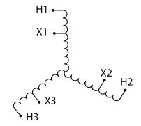
Three Phase Encapsulated Autotransformer with a capacity of 112.5kVA, transforming 600Y Volts to 480Y Volts
