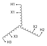
Three Phase Autotransformer with a capacity of 30kVA, transforming 415Y Volts to 110Y Volts
