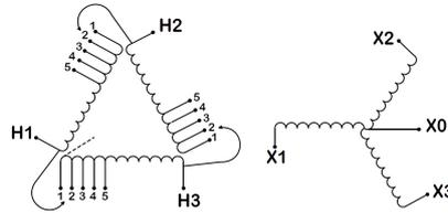
Three Phase Encapsulated Isolation Transformer with a capacity of 112.5kVA, transforming 480 Volts to 380Y/220 Volts
