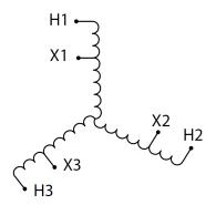
Three Phase Autotransformer with a capacity of 450kVA, transforming 416Y Volts to 277Y Volts
