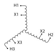
Three Phase Autotransformer with a capacity of 600kVA, transforming 416Y Volts to 380Y Volts
