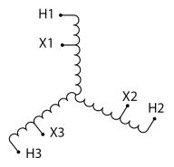
Three Phase Autotransformer with a capacity of 300kVA, transforming 600Y Volts to 208Y Volts
