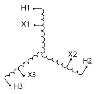
Three Phase Autotransformer with a capacity of 600kVA, transforming 600Y Volts to 416Y Volts
