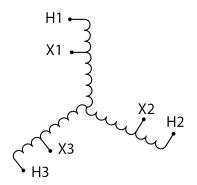
Three Phase Autotransformer with a capacity of 500kVA, transforming 230Y Volts to 347Y Volts
