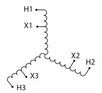
Three Phase Autotransformer with a capacity of 6kVA, transforming 440Y Volts to 400Y Volts
