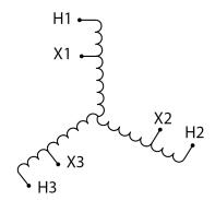
Three Phase Autotransformer with a capacity of 150kVA, transforming 220Y Volts to 110Y Volts
