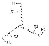
Three Phase Autotransformer with a capacity of 300kVA, transforming 400Y Volts to 220Y Volts
