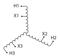
Three Phase Autotransformer with a capacity of 600kVA, transforming 200Y Volts to 440Y Volts
