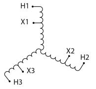
Three Phase Autotransformer with a capacity of 600kVA, transforming 347Y Volts to 440Y Volts
