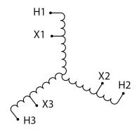
Three Phase Autotransformer with a capacity of 750kVA, transforming 277Y Volts to 550Y Volts
