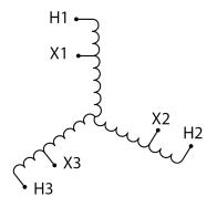
Three Phase Autotransformer with a capacity of 15kVA, transforming 347Y Volts to 110Y Volts
