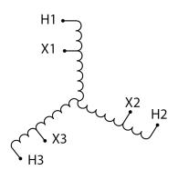
Three Phase Autotransformer with a capacity of 750kVA, transforming 380Y Volts to 575Y Volts
