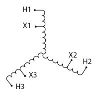
Three Phase Autotransformer with a capacity of 150kVA, transforming 416Y Volts to 115Y Volts
