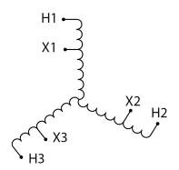
Three Phase Autotransformer with a capacity of 45kVA, transforming 380Y Volts to 347Y Volts
