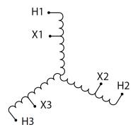
Three Phase Autotransformer with a capacity of 2500kVA, transforming 277Y Volts to 208Y Volts
