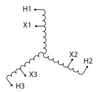
Three Phase Autotransformer with a capacity of 500kVA, transforming 600Y Volts to 440Y Volts
