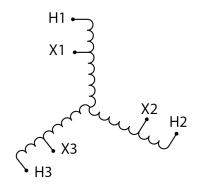
Three Phase Autotransformer with a capacity of 225kVA, transforming 400Y Volts to 200Y Volts
